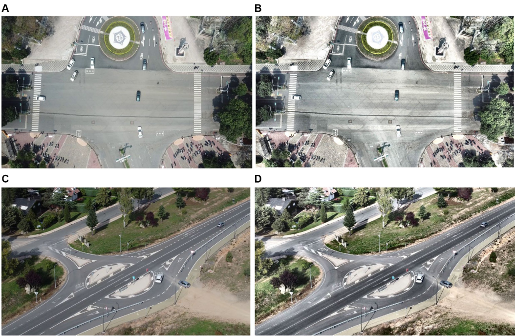
FIGURE 2 Defogging results over the (A) original image of VEDAI dataset (B) defogged image (C) original image of SRTID dataset (D) defogged image.
