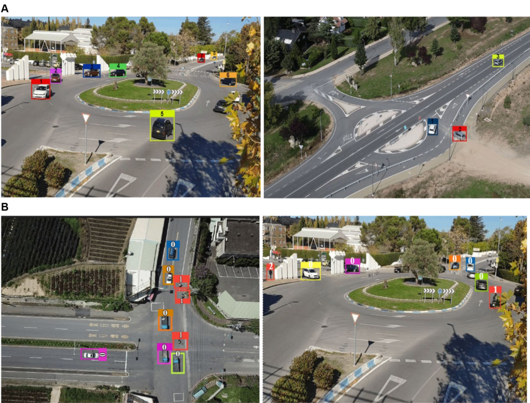
FIGURE 10 Tracking results using DeepSORT tracker across the image frames (A) Vehicle detection only (B). Multiple-object detection (0 = Vehicles, 1 = Bike, 2 = Pedestrians in frames).
