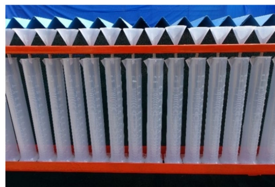
FIGURE 8 Arrangement of measuring jar in spray patternator.
