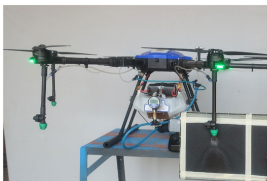
FIGURE 6 Experimental layout for measurement of spray angle.
