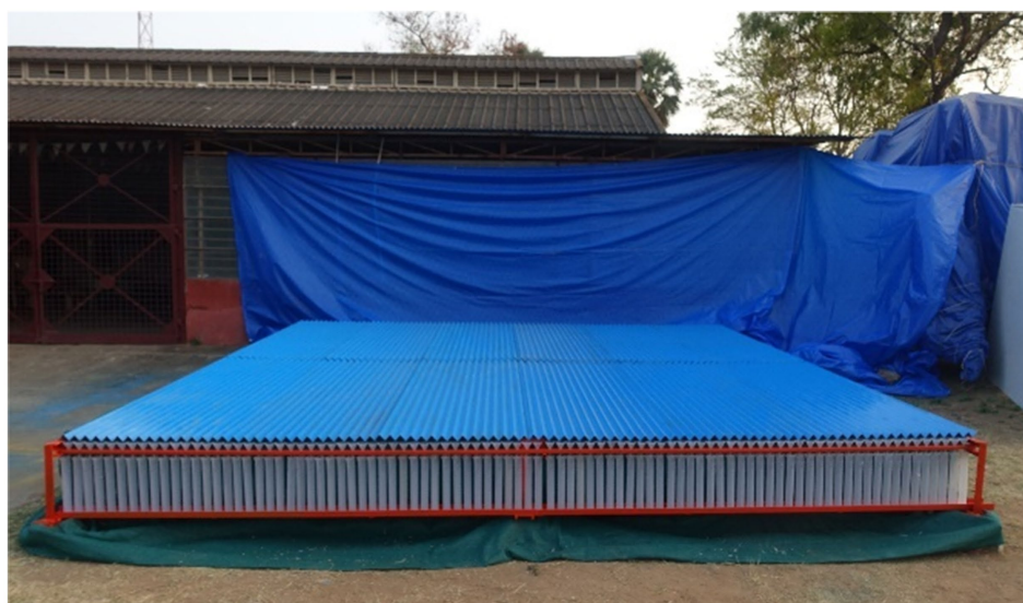
FIGURE 10 Developed spray patternator for spray volume distribution measurement.
