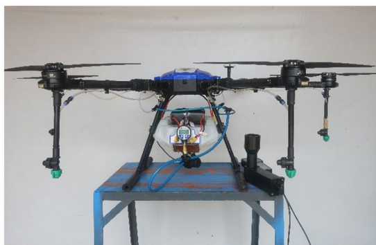
FIGURE 4 Experimental layout for measurement of spray discharge rate using nozzle tester.
