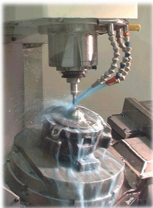
FIGURE 2 | Coolant applied during machining finishing of the cup after porous coating.
