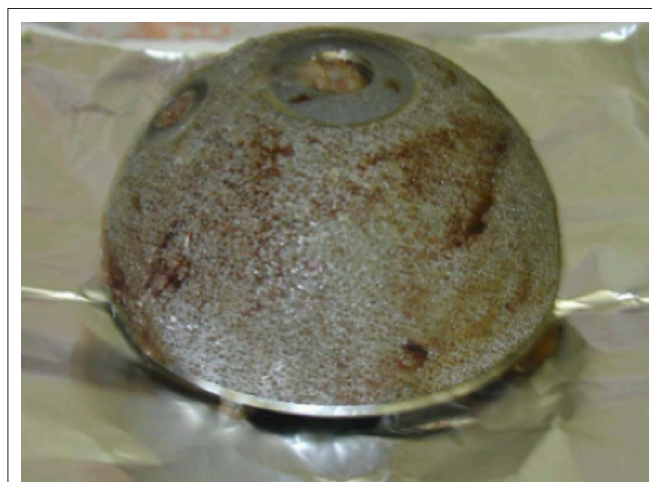
FIGURE 1 | Revised Inter-Op cup after 11 months in vivo showing no bone ingrowth and a few areas with a red and gray gel-like residue.
