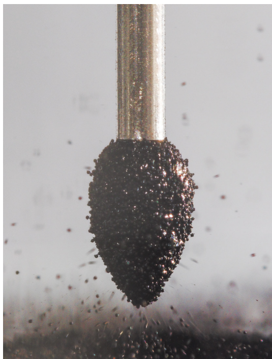
"Polypyrrole coated polystyrene particles attracted electrostatically to a pendent water drop" by Eddie O'Reilly is licensed under CC-BY.
