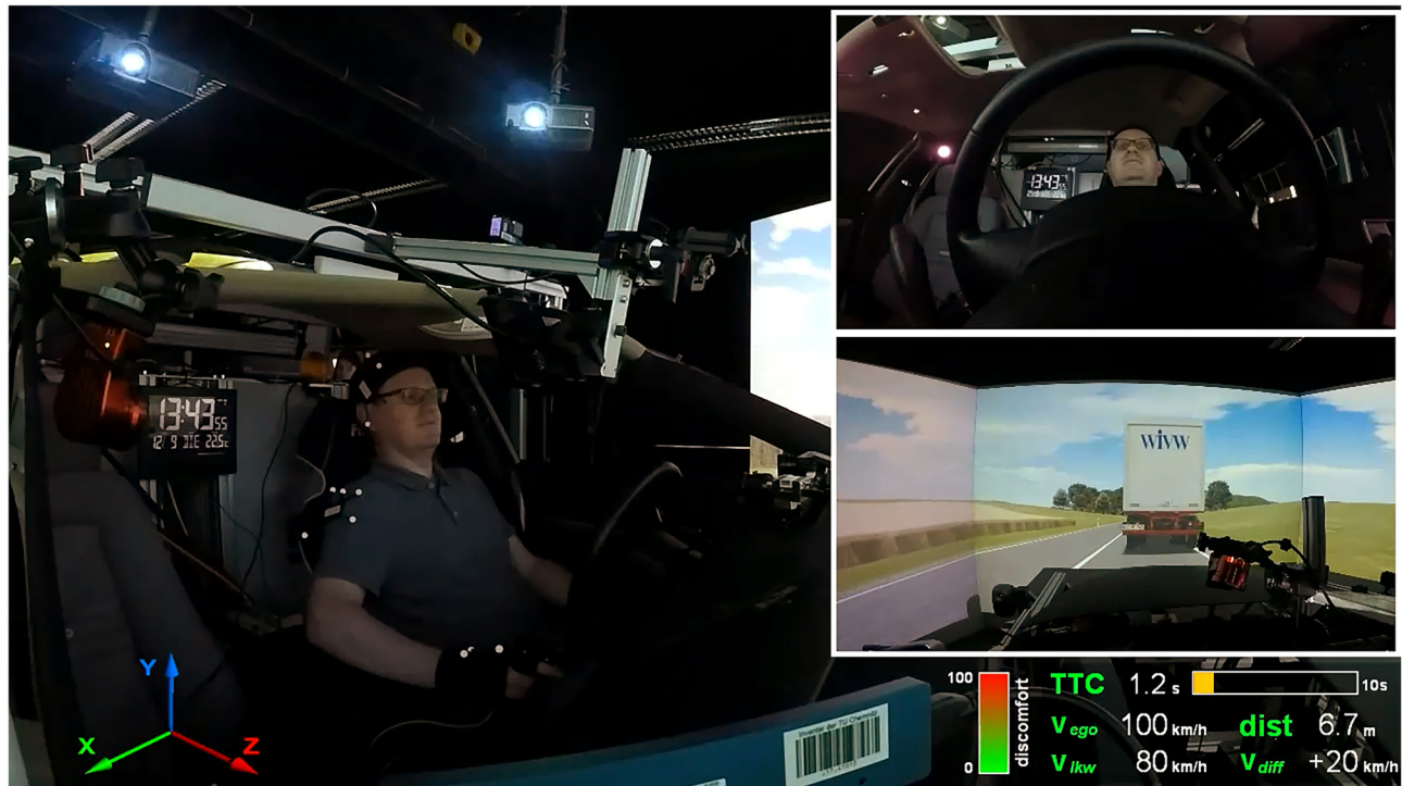
FIGURE 1 | Setup of the driving simulator study during one approach situation to the truck driving ahead. Left side: motion capture markers at head, right shoulder, and hands; handset control for reporting discomfort held in the right hand. Right side: driver camera view (top); front scenery camera view recorded from the roof of the mock-up (middle); reported discomfort as well as driving parameters at that particular moment such as TTC, ego speed/truck speed/speed difference and distance to the truck (bottom). Written informed consent was obtained from the individual for the publication of this image.
