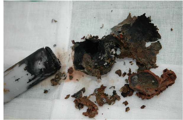
FIGURE 7 | Implant (Telonics IMP/400/L, 15.2 × 3.3 cm) removed from a 6-years old female bear (BD124) that had carried the device for 5 years. The batteries had short-circuited, with subsequent over-heating of the device and leakage from the batteries. One end cap was detached and the outside of the implant was partly covered by a soot-like material. All internal components appeared to be burned and were covered by the same soot.
