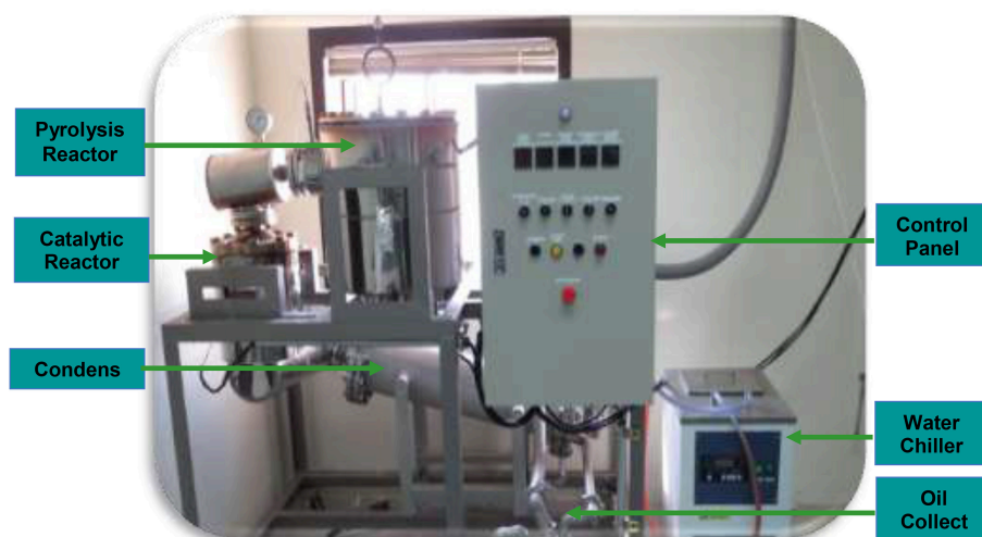
FIGURE 1 | Small pilot scale pyrolysis reactor (Miandad et al., 2016b).
