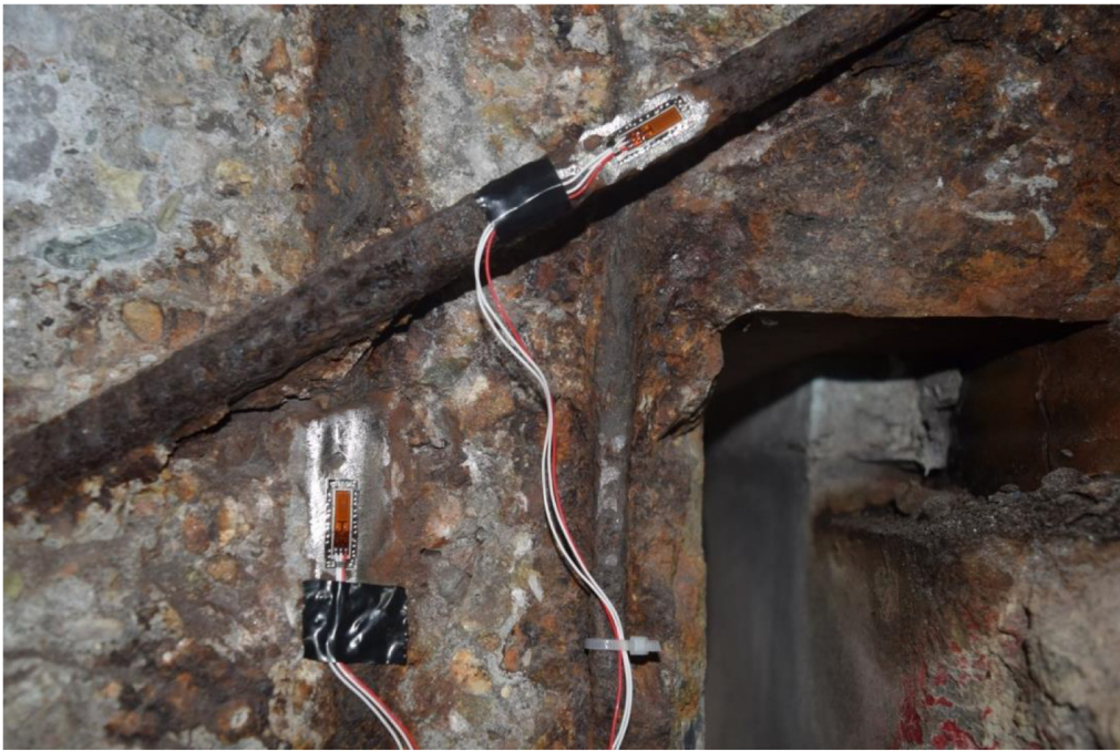
FIGURE 6 | Weldable strain gauges on exposed rebars at dapped end.
