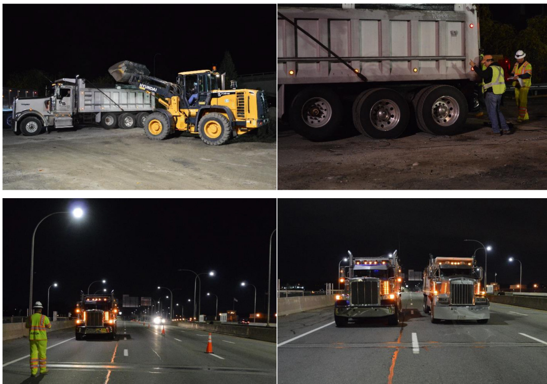
FIGURE 9 | Photos of loading and weighing test trucks and operating test runs.
