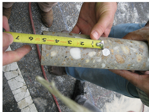
FIGURE 4 | Cylindrical concrete sample drilled (1 inch = 25.4 mm).
