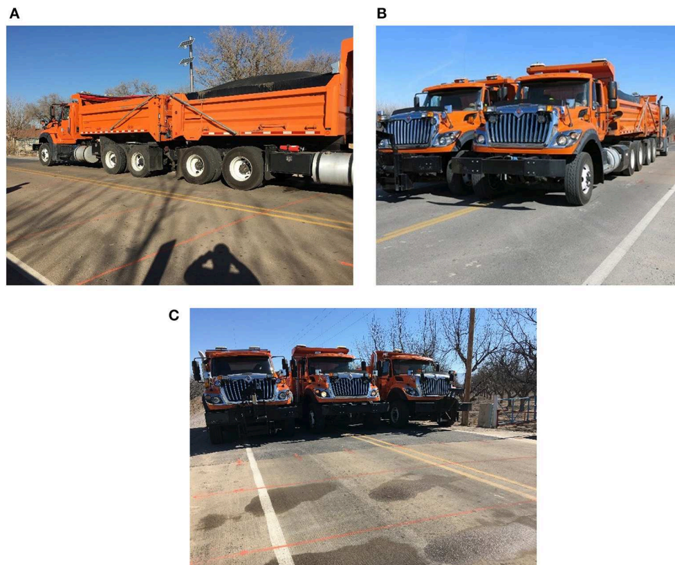
FIGURE 7 | (A) Single truck back-to-back loading, (B) double truck back-to-back loading, (C) triple truck side-by-side loading.
