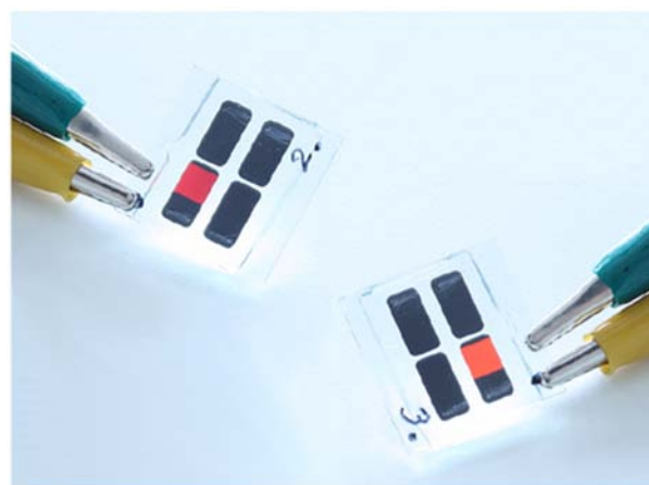
FIGURE 4 | Photographs of the multicolor light emitting diodes utilizing the size-separated silicon nanocrystals prepared by the thermal process of the sol-gel precursor (hydrogen silsesquioxane). Reprinted with permission from Maier-Flaig et al. (2013), Copyright 2013 ACS Publishing.
