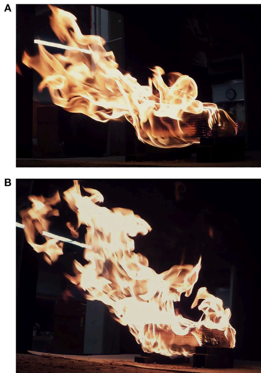
FIGURE 10 | Crib design #22 in 0.7 m/s (A) and 0.24 m/s (B) wind from behind demonstrating flames hugging the top and bottom sides of the fuel bed, blocking airflow from below.
