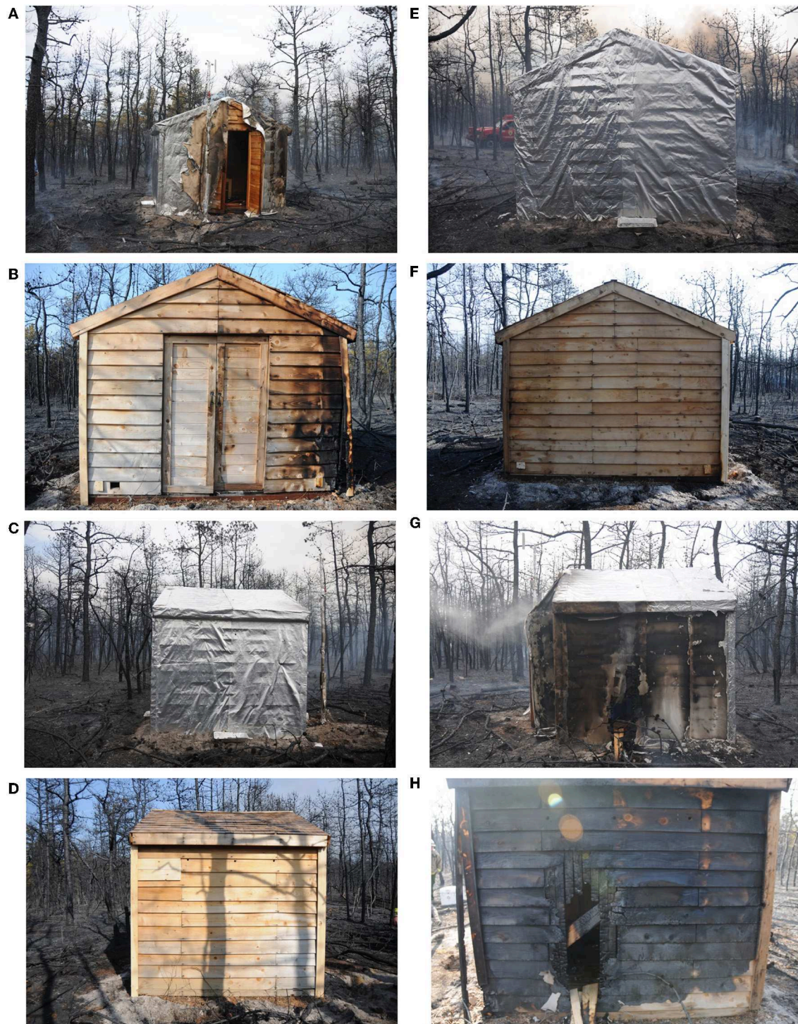
FIGURE 10 | Fire blanket and wood structure damage after the prescribed burn (see Table 4 for the blanket materials). (A,B) Wall "A" facing south, (C,D) Wall "B" facing west, (E,F) Wall "C" facing north, and (G,H) Wall "D" facing east.
