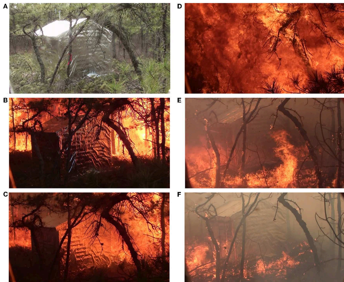
FIGURE 9 | Video images from the northeast side captured the fire front approaching from the east side and passing over the blanketed wood structure in a few minutes (see Supplementary Video 3 ). (A) The fire front is still ~20 m away, (B) approaching, (C) arriving, (D) engulfing, (E) passing the shed, and (F) additional fuels continue to burn.
