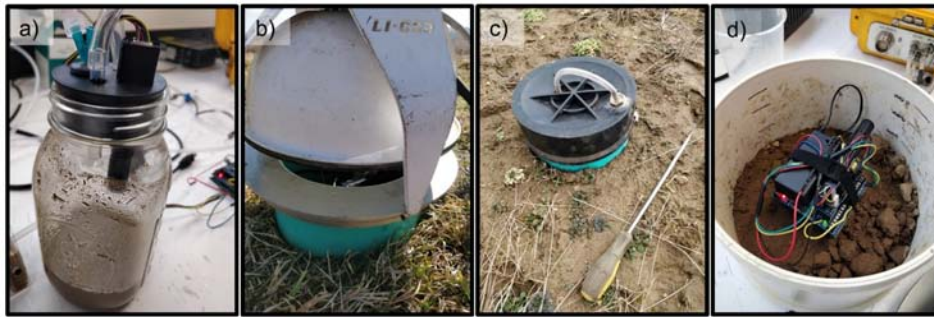
FIGURE 2 | Measurement setups for: (a) SMAAC-Biomass substrate induced respiration (SIR) measurement; (b) SMAAC-Field flux measurement with SMAAC simultaneously located within the LI-COR 8100 sampling chamber; (c) SMAAC-Field flux measurement with SMAAC independent of the LI-COR unit; and (d) SMAAC-Burst laboratory CO 2 burst measurement.
