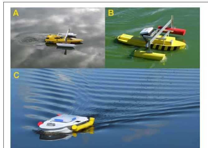
FIGURE 2 | Design iterations of the sonar profiling ROV (detailed specifications in Table 1 ). (A) The prototype was an off-the-shelf speed boat, fitted with a frame to mount the sonar unit and stabilizers to the boat. (B) Redesign of the boat with a more robust deep V-shaped hull, with frame for sonar and stabilizers. (C) Current boat design with U-shaped hull and sonar mounted inside.
