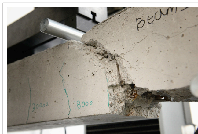
FIGURE 7 | Bamboo composite reinforced concrete beam after failure.
