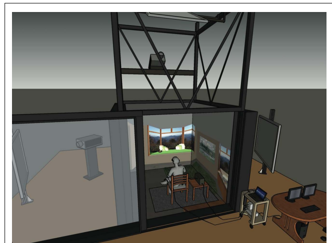
FIGURE 1 | Schematic of the control room and Duke's immersive virtual environment (DiVE) with a human participant viewing a virtual scene.
