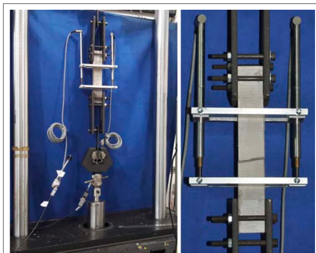
FIGURE 3 | Assembling the tensile strength test and fractured specimen.
