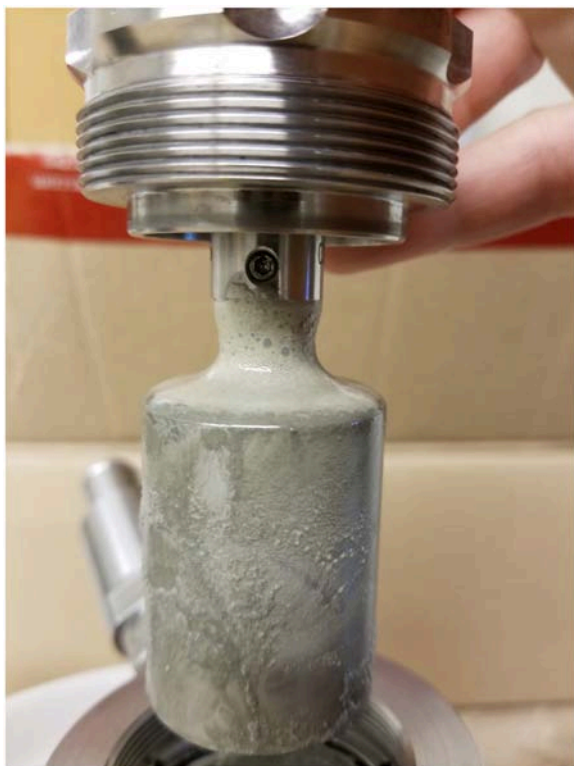
FIGURE 5 | The pressurization/depressurization of the samples yielded a substantial volume of foam on top of the inner cylinder of the pressure cell. Picture taken after removing the inner cylinder from the pressure cell.
