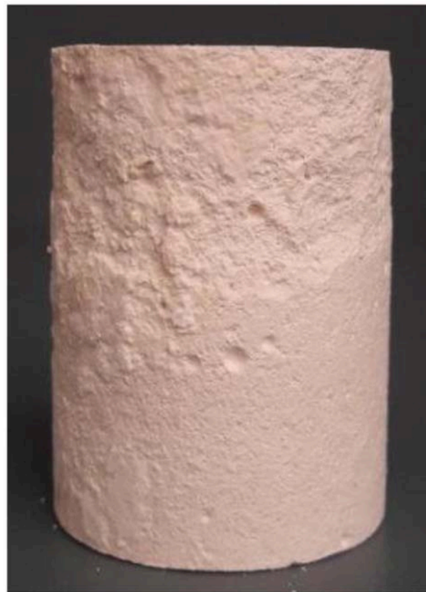
FIGURE 9 | Sample with calcined kaolin as precursor and activated with 10% of Na 2 O from NaOH with visible surface deterioration.
