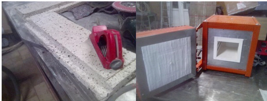
FIGURE 12 | The processing of prepared AAM plates with simple tools (a) and created prototype of high temperature oven.
