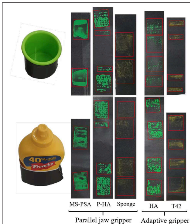
FIGURE 15 | Example of identification and comparison of contact areas for different types of hands and grippers grasping two different objects: a small cup ( Top ) and a bottle of mustard ( Bottom ). Green acrylic paint was applied to the finger-pads of the examined robot grippers and hands while yellow chalk was applied onto the sponge and T42 gripper finger-pads (maintains better contact). The red boxes enclose the estimated surface areas of the contact patches during grasping. The results demonstrate that for grasping the mustard container, the sponge had the largest surface contact area, followed by HA, T42, P-HA, and MS-PSA gripper. While grasping a smaller and lighter cup, the HA gripper had the largest contact area followed by the parallel jaw HA, parallel sponge, and MS-PSA gripper. T42 had the least contact surface with the object.
