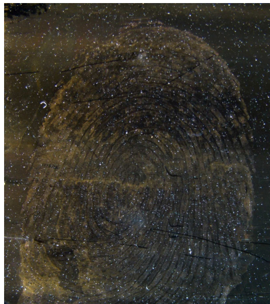
FIGURE 3 | Stereomicroscopy image (5 \times objective) of a complete SMD revealed fingerprint on a glass substrate.
