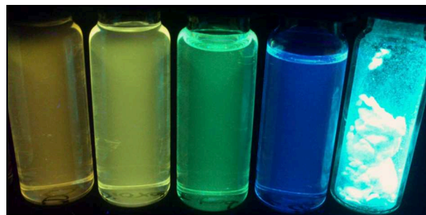
FIGURE 8 | Dyad 5a in the solid state and in cyclohexane, toluene, 1,4-dioxane, and dichloromethane solutions (from left to right) under a handheld UV lamp (λ exc = 365 nm).
