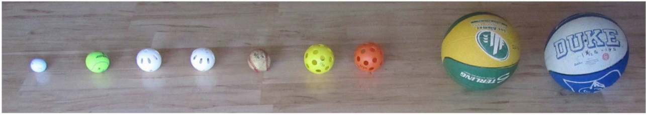
FIGURE 2 | The balls that were dropped from the bridge, with the volleyball omitted. From left to right: Golf Ball, Tennis Ball, Whiffle Ball 1, Whiffle Ball 2, Baseball, Yellow Whiffle Ball, Orange Whiffle Ball, Green Basketball, and Blue Basketball. The two colored whiffle balls have circular openings and are structurally identical. The two white whiffle balls have elongated slits and are also identical.
