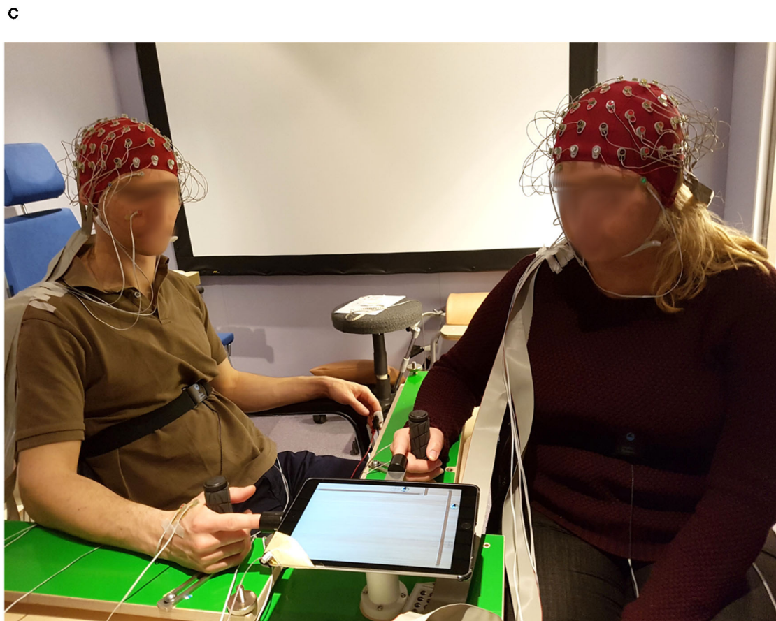
FIGURE 1 | Target tracking task in the collaborative ( A ) and individual condition ( B ). Dashed lines visualize the trajectory of the target; they were not visible to the subjects. The picture ( C ) shows the experimental setup and two participants with EEG caps.
