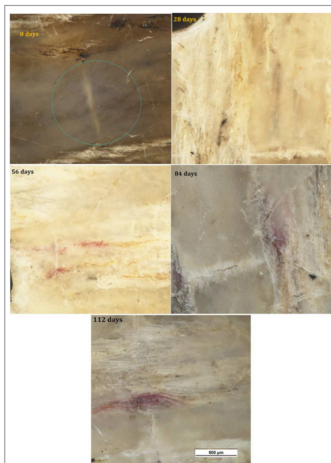
FIGURE 7 | Optical micrographs of PHBV/PBAT/flax at 0, 28, 84, and 112 days.
