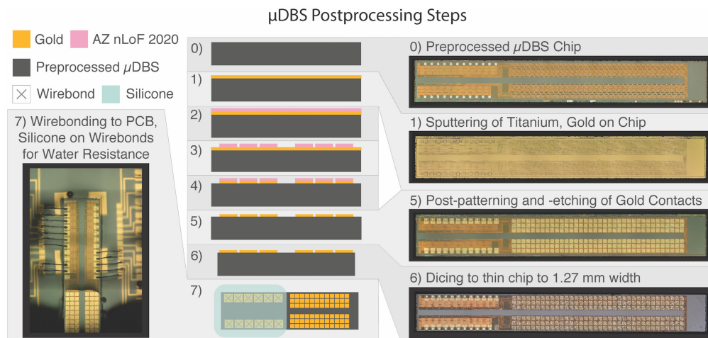
FIGURE 3 | Design architecture for \mu DBS post-processing. Fabricated chips (0) undergo gold deposition (1) and are covered with AZ nLoF 2020 negative photoresist (2). Photoresist is exposed to UV light according to the desired contact layout through a photolithography mask and regions of photoresist not exposed to light are removed (3). Gold and titanium layers are etched away from regions not covered by photoresist to define the gold contacts (4). Remaining photoresist is washed off (5) and the chips are diced to the appropriate size (6). Connection pads are wirebonded to test PCBs (7) to enable device programming and functionality testing. Silicone was used to insulate non-contact regions from water exposure during the validation experiments.
