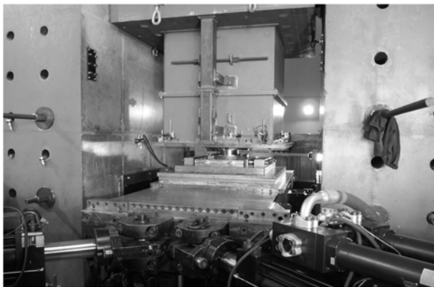
FIGURE 3 | Testing setup of the Bearing Tester System at the EUCENTRE Foundation.
