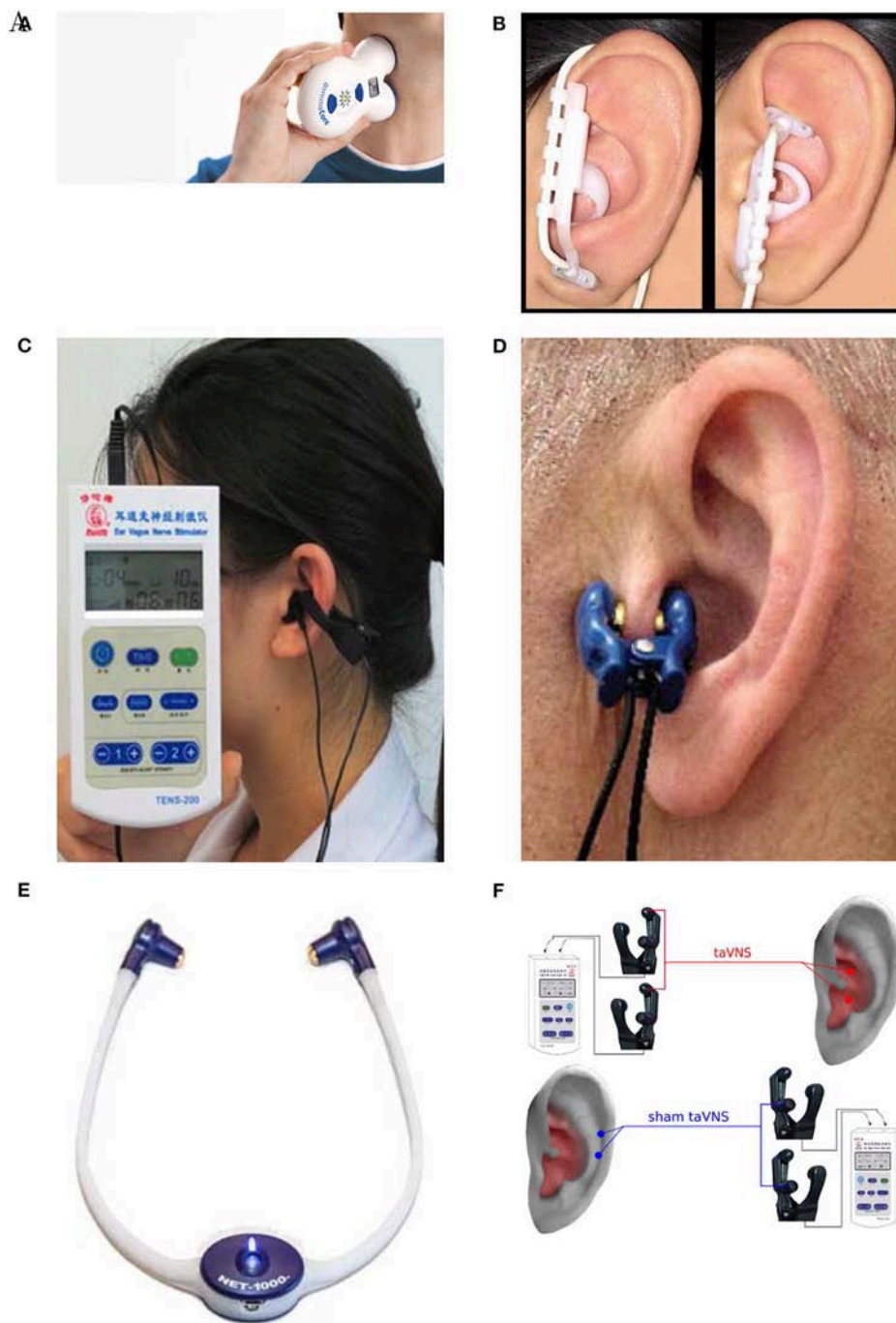
FIGURE 5 | Stimulation electrode positions. (A) Neck stimulation using a gammaCore device (Silberstein et al., 2016b). Image courtesy of electroCore Inc, electrocore.com. (B) Earlobe sham and cymba concha stimulation using NEMOS electrodes (Frangos et al., 2015). (C) External ear canal and concha stimulation using a TENS device from Suzhou (Liu et al., 2018). (D) Tragus stimulation (Lehtimäki et al., 2013). (E) External ear canal stimulation using a headset NET-1000 (Hein et al., 2012). Image courtesy of Auri-Stim Medical Inc, net1device.com. (F) Concha and cymba concha active stimulation (Rong et al., 2016). All figures reproduced with permission.
