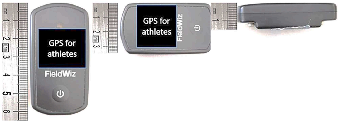
FIGURE 1 | Details of the GNSS Sensor; dimensions: 65 × 35 × 15 mm; weight: 35 g.
