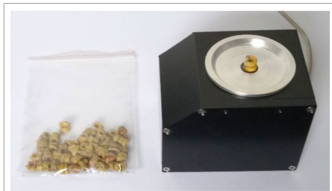
FIGURE 3 | The sample presentation to record NIR spectra of fengdous.
