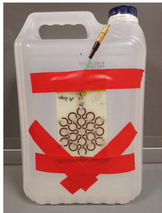
FIGURE 2 | Photograph of the phantom with the 7 T MLC attached to it.
