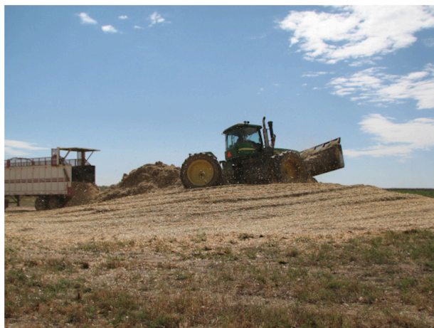
FIGURE 8 | Simultaneous formation and compaction of a drive over storage pile with corn stover unloaded from walking floor trailers.
