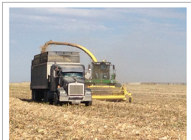
FIGURE 7 | Collection of corn stover with forage chopper into a walking floor trailer.
